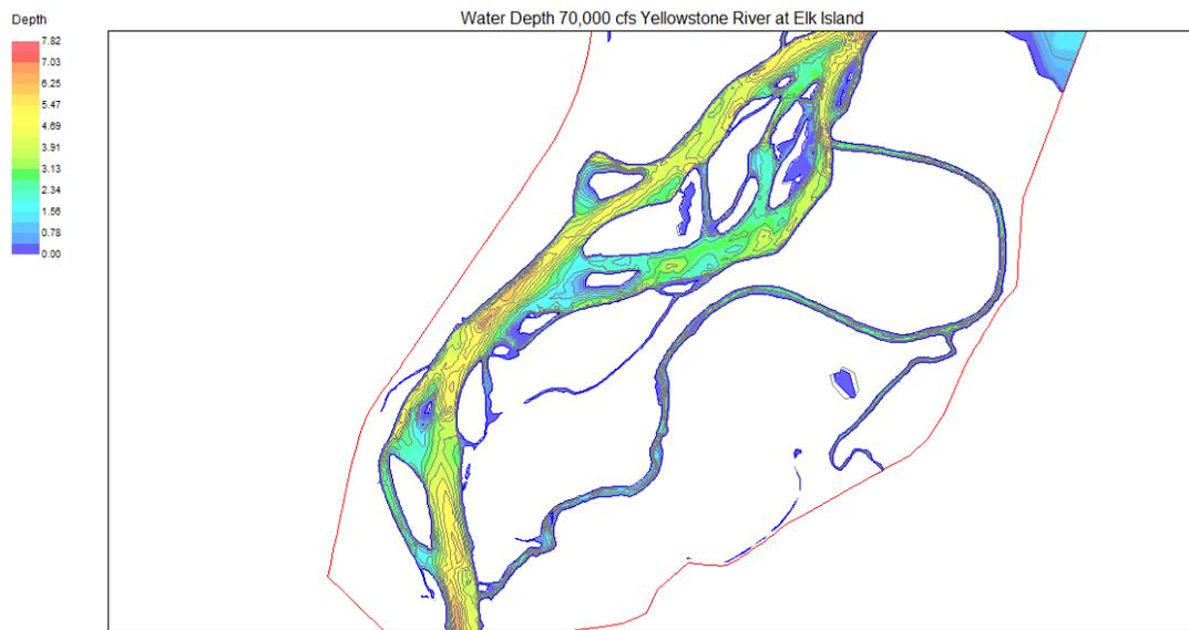
Figure 5. Example of 2-D model depth contours.
