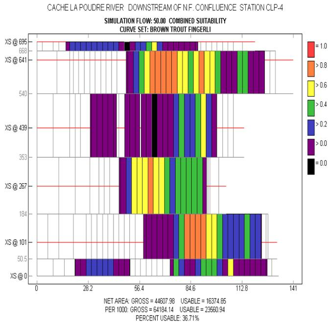
Figure 1. One-dimensional model representation of river channel (units for X and Y axis are in feet, legend on right side y axis is decimal weighting factor.)
