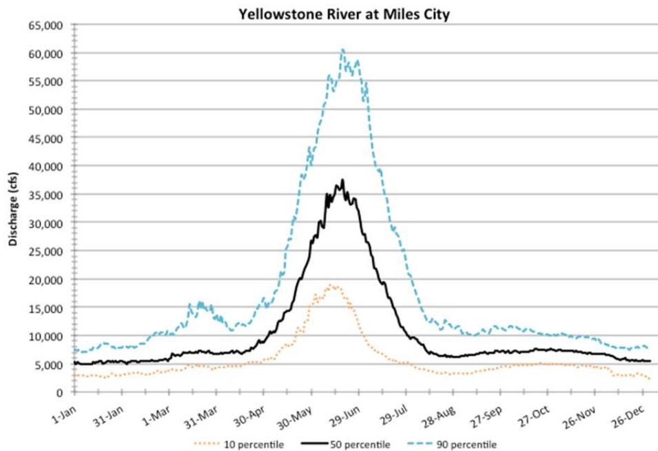
Figure 8. USGS 06309000 Yellowstone River at Miles City MT, flow exceedence percentiles for the period of record 1923 – 2012.
